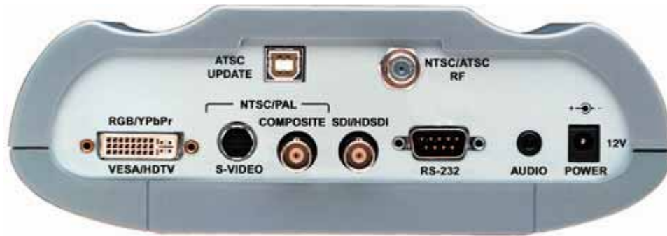
Figure 3. The SDI/HDSDI output of the Sencore VideoPro provides standard SDI or HDSDI signals through a standard BNC interface connection.
