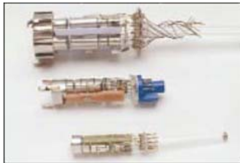
Fig. 1 - Today's electronic guns have gotten smaller and are capable of producing better quality pictures.
