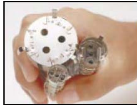
Fig. 2 - Sizes of CRT's have changed dramatically over the years from the old Delta gun style to today's newest in-line. The smaller in-line gun produces much better convergence.
