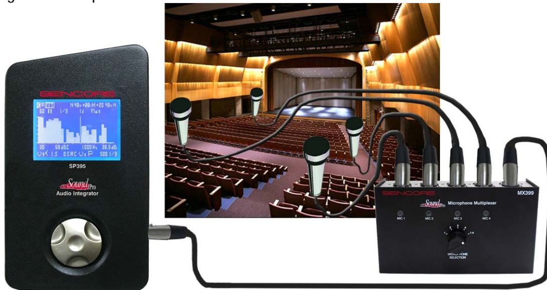
Figure 3. Multiplexing microphones placed throughout the listening position provides a single continuous active average measurement of the room's frequency response at all listening positions.
