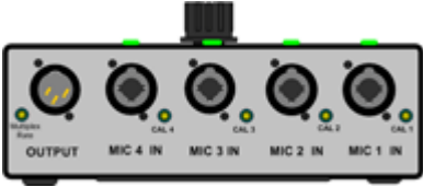
Figure 3. Calibration controls on each microphone input provides level adjustment for accurate measurements.
